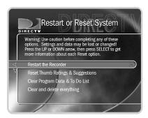
If you do not have the remote control, you can also press buttons on the front of the DVR to enter the safety code. Press the INFO button three times and then press DOWN.
